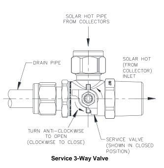
• The mains pressure will force water to flow from the tank and through the pipe work, forcing air from the collector circuit through the service valve. This is evidenced by spurting of water from the drain line connected to the service valve.
