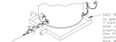
SAFE TRAY WITH DRAIN As specified in AS/NZS 3500.4 If there is likelihood of leaking water causing damage to property (carpets,furniture,etc) then fitting a Safe Tray is recommended. Note: Manufacturer's warranty does not cover property damage.
