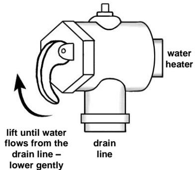
If water does not flow freely from the drain line when the lever is lifted, then the water heater must be checked. Phone Rheem Service or their nearest Accredited Service Agent / Centre to arrange for an inspection.
