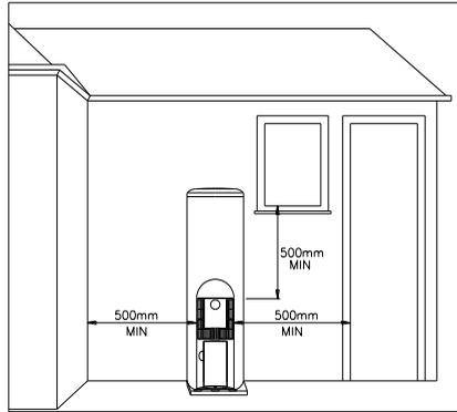
**Note:** \* If these horizontal distances cannot be achieved, AS/NZS 5601.1 states an equivalent horizontal distance measured diagonally from the nearest discharge point of the flue terminal to the opening may be deemed to comply. Check with the local regulator.
