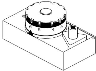
To increase the water temperature to 65°C, turn the gas control knob anticlockwise to a setting of '7'. Refer to [“Hotter Water Increases the Risk of Scald Injury”](#) on page 10.
