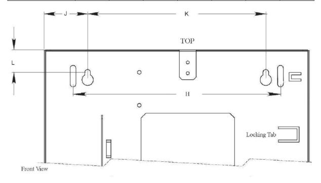
Note: - measurement 'H' only applicable to 3 & 5 litre models. Slots do not appear on larger model back plates.
