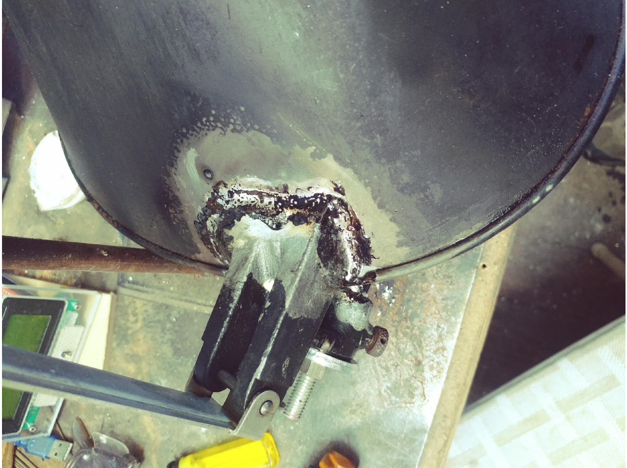
Fig. 10: closeup of top joint post-soldering.
