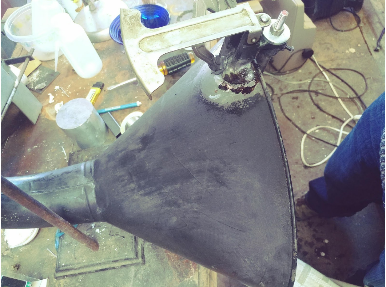
Fig. 9: bracket clamped to horn, first solder joint finished. Flux debris is visible across the joint.
