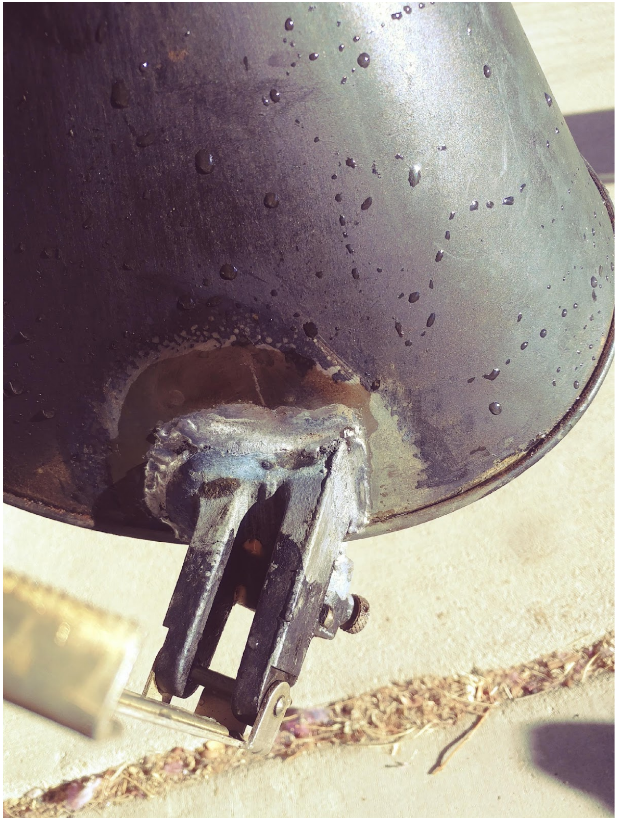
Fig. 11: soldered, washed, and wire brushed.
