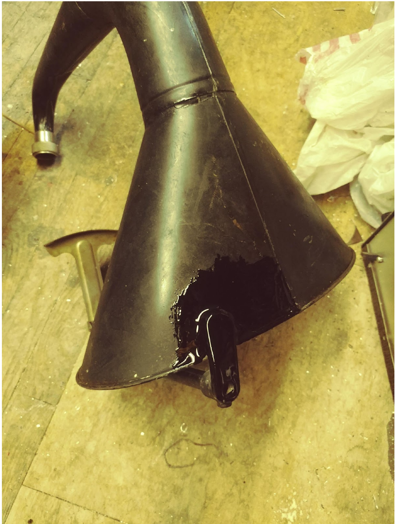
Fig 16: Japanning applied, thick viscous coat slowly drying.
