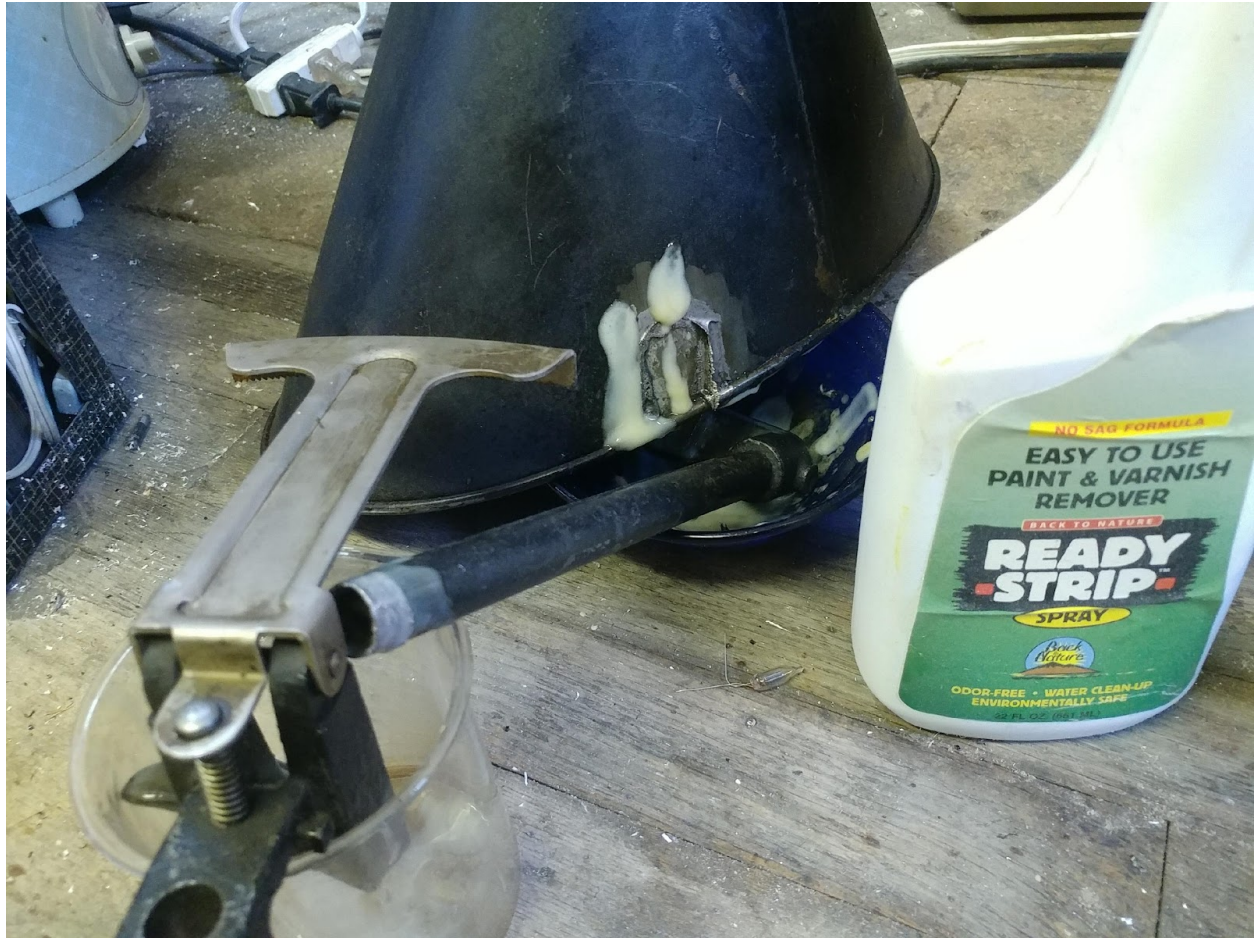
Fig. 7: starting the process of stripping off the coating.
