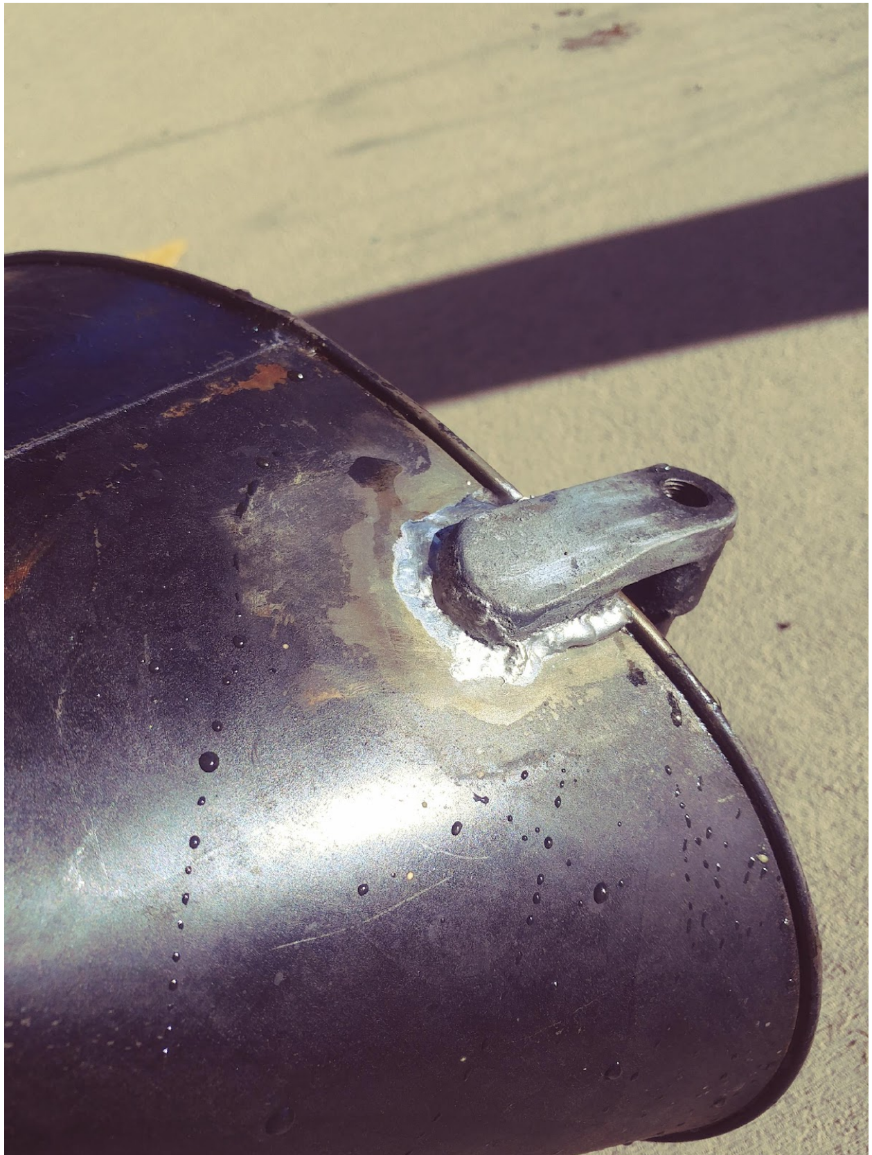
Fig. 12: lower bracket soldered, washed, cleaned up.
