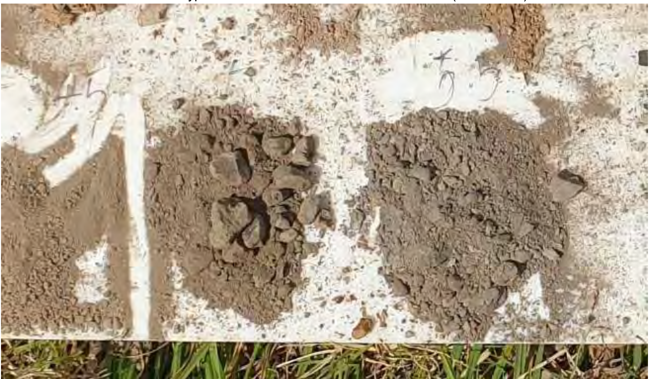
Photo 6 - Typical BEDROCK unit encountered in BH08 (21/02/2022)
