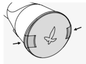
To remove the cap, press together the protruding snap elements at the rim of the cap.
