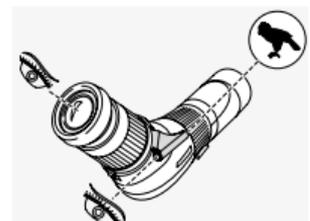
The mounted aiming aid is designed to help you align the spotting scope with the subject to be observed.
