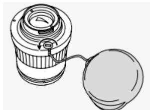
The protective cap for the eyepiece is attached to the eyepiece with a cord. By loosening the screw on the eyepiece with a screwdriver, you can remove the cord with the cap from the eyepiece. Please reinsert the screw.
