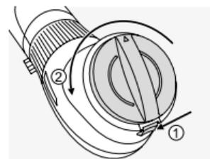
To remove the cover, slide the locking mechanism of the eyepiece downward and turn the protective cover to the left (counterclockwise).
