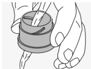
The housing is best cleansed with a soft, moist cloth (don't use the lens-cleaning cloth).
