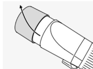
The integrated, extendable sunshield keeps away disturbing lateral light and protects the objective lens from rain. The sunshield is best slid out and in with a slight rotary motion.
