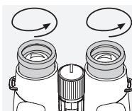
**Pos. A:** Initial position without eyeglasses: For this, twist out the eyecups counterclockwise to the full extent.
