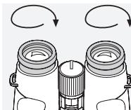
**Pos. B:** Initial position with eyeglasses: Twist in the eyecups clockwise until they stop.
