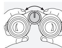
It is possible to bring every subject into focus from the shortest adjustment distance (see technical data sheet) to infinity by turning the focusing wheel.
