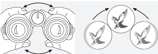
To see a single round image, turn the two halves of the binoculars until no irritating shadows can be seen.
