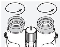
**Pos. A:** Initial position without eyeglasses: For this, twist out the eyecups counterclockwise to the full extent.
