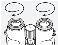
**Pos. C and D:** Alternative positions or interim adjustment stages for eyeglass-wearers and non-eyeglass-wearers.
