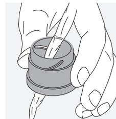
**Cleaning the protective housing.** Use the soap & brush kit (supplied). Close the covers on the eyepiece and objective lenses. Moisten the brush and apply the soap using circular movements to gently clean the housing. Rinse the binoculars with clean water and dry with care. If the optics become wet,
