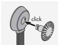
Align the button pin with the strap connector ring and press until it clicks.
