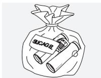
Keep your binoculars in their bag in a well-ventilated place. If the binoculars are wet, they must be dried first.
