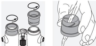
**Cleaning the protective housing.** Use the soap & brush kit (supplied). Close the covers on the eyepiece and objective lenses. Moisten the brush and apply the soap using circular movements to gently clean the housing. Rinse the binoculars with clean water and dry with care. If the optics become wet, dab them dry with a clean cloth to prevent scratching. Rinse the brush thoroughly and leave the soap & brush kit to dry.
