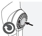
Press the pin in firmly and turn slightly clockwise until it clicks.
