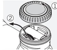
1. Open the battery cover and remove the torx wrench and the adjusting tool.
