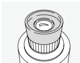
By turning back the eye-cups, the eyeglass-wearer can optimally utilize the full field of view. The eyecups can be unscrewed for cleaning or replacement.
