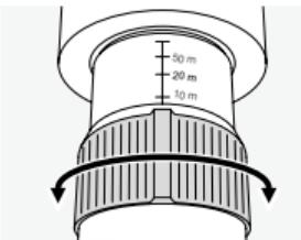
On the ocular you find a scale for the estimation of distance. This scale is designed for easy focusing.
