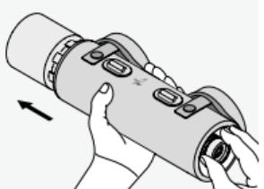
As the stay-on case size is perfectly sized to fit your spotting scope a slight adherent-effect between the stay-on case and the spotting scope may occur through time. Removing the stay-on case can best be achieved by holding the spotting scope with one hand and pushing the extendable spotting scope from the eyepiece side forwards out of the stay-on case.
