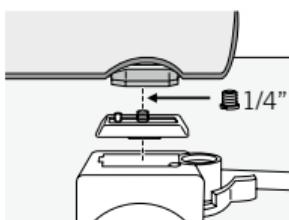
The tripod base has a connecting thread of 3/8" UNC. The inserted bush reduces the connecting thread to 1/4". The spotting scope thus fits on any standard tripod.
