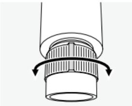
By turning the ocular you can focus any object sharply at a distance of 10 m / 33 ft to infinity. In the infinity position the nose on the ocular is at the top.
