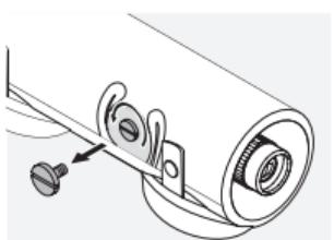
The tripod base has a connecting thread of 3/8" UNC. The inserted bush reduces the connecting thread to 1/4". The spotting scope thus fits on any standard tripod.
