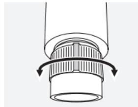
By turning the ocular you can focus any object sharply at a distance of 10 m / 33 ft to infinity. In the infinity position the nose on the ocular is at the top.
