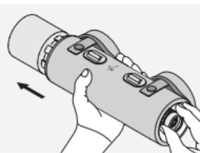
As the stay-on case size is perfectly sized to fit your spotting scope a slight adherent-effect between the stay-on case and the spotting scope may occur through time. Removing the stay-on case can best be achieved by holding the spotting scope with one hand and pushing the extendable spotting scope from the eyepiece side forwards out of the stay-on case.
