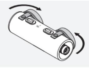
The spotting scope is placed in a stay-on case. The caps of the stay-on case can be pushed to the side (without opening the press studs) for observing. Alternatively, you can open one of the press studs, move the caps to the side of the body and then close the press stud again.
