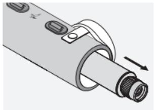
Hold the body and the ocular of the spotting scope firmly and then pull outwards until the extension reaches its stopping point.
