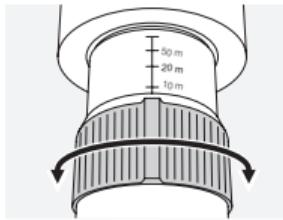
On the ocular you find a scale for the estimation of distance. This scale is designed for easy focusing.
