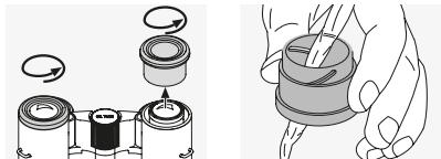
In the event of hard-to-remove dirt (e.g. sand) the eye cups can be unscrewed and cleaned easily.
