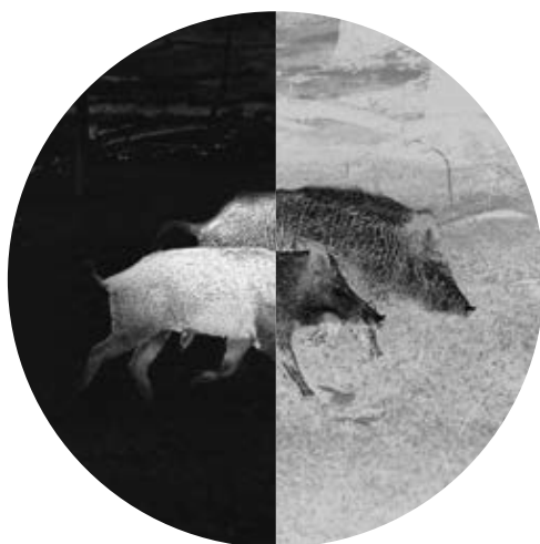
Thermal image display in two modes: left white-hot (white heat sources), right black-hot (black heat sources)
