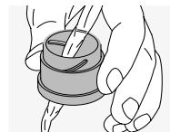
In the event of hard-to-remove dirt (e.g. sand) the eye cups can be unscrewed and cleaned easily.
