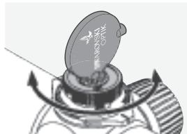
Sight in the elevation by turning the top section of the dial as shown in figure 01. If you are sighting in at 100 yards, turn to the right or left until your elevation is dead on at 100 yards. This will become the zero setting during further assembly. To do this, turn the upper detent ring in the required direction. Use the coin opener if necessary.
