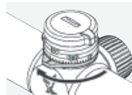
Close the locking mechanism after using the ballistic turret to avoid unintentional re-adjustment by turning the locking ring clockwise a quarter turn.
