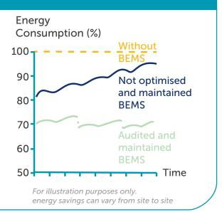
system can reduce most buildings' energy and carbon by 20%. However, if left, over time this saving gets lost as setpoints and timers get changed, or worse, plant is set to manual and always on.
