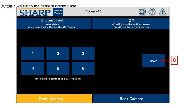
The camera preset page will recall a saved preset or allow a currently positioned camera to be saved as a preset. After positioning a camera press and hold a preset button for 3 seconds to save that position.
