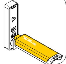
While the LED is flashing, insert the Programming Key.
