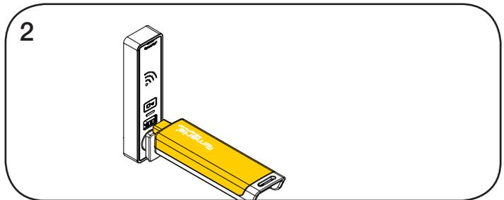
2 While the LED is flashing, insert the Programming Key.
