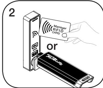
2 While the LED is flashing, insert a valid Manager Key or present a valid Manager RFID.
