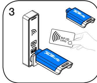
3 While the LED is on, insert each User Key or present each User RFID one at a time.
