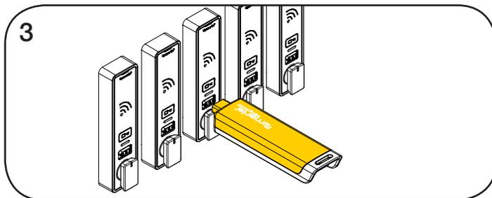
Insert the Programming Key to program each lock to operate with the same Manager Credentials.
