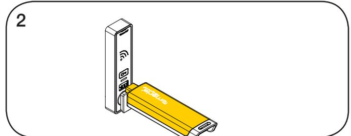
While the LED is flashing, insert the Programming Key. A two-tone beep will be heard and the LED will turn off.
