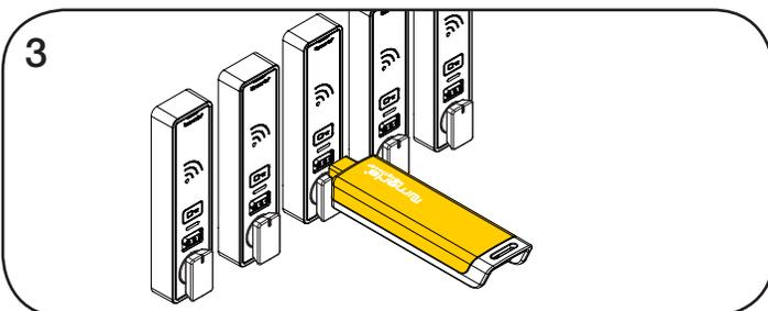
3 Insert the Programming Key to program each lock to operate with the same user and manager credentials.
