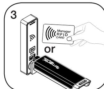
While the LED is flashing, insert each additional Manager Key or present each RFID Credential one at a time.
