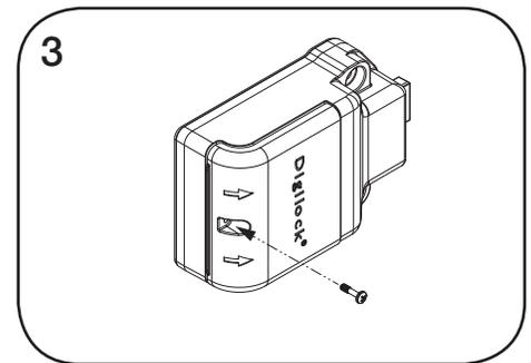
3 Replace the Cover Plate and secure with the screw.
