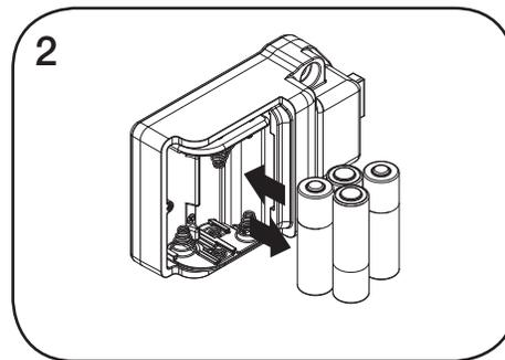
2 Remove the batteries from the housing.
