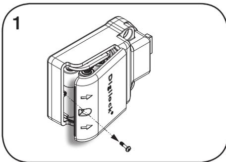
1 Remove the screw from the Cover Plate with a Phillips head screwdriver.
