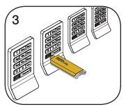
Insert the Programming Key to program each lock to operate with the same user credentials and Manager Keys.
