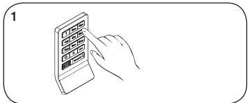
Go to a lock already programmed to operate with the Manager Keys. Press © 🚾 6 1 🚾.
