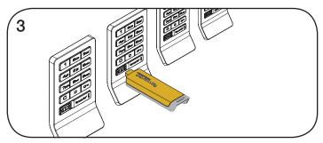
Insert the Programming Key to program each lock to operate with the same Manager Keys.
