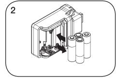
Remove the batteries from the housing.
