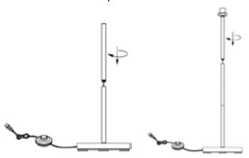
STEP 4. Squeeze the Support Bar (C) and slide it into the base as shown.
