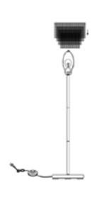
STEP 7. Screw the Decorative cap back onto the Support Bar (C) over the Shade (A) as shown.
