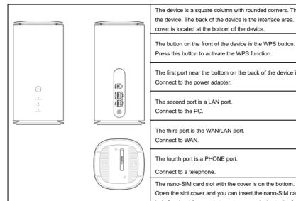
The device is a square column with rounded corners. There is a button on the front of the device. The back of the device is the interface area. The nano-SIM card slot with the
