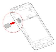
Hold the microSDXC card with the cut corner oriented as shown and slin it into the card slot
