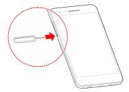
Pull out the card tray. You can place a nano-SIM card on the right card slot, and place a microSD card on the left card slot, as shown. Carefully slide the tray back into place.
