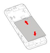
4. Install the back cover in the order and direction as shown in the figure.
