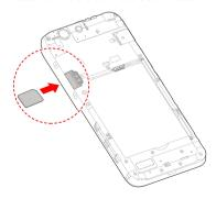
► Hold the microSDXC card with the cut corner oriented as shown and slip it into the card slot.
