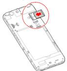
Insert the battery. Make sure the connectors on the battery go into the battery compartment first and align with the connectors in it. Gently push down on the battery until it clicks into place.
