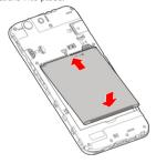
Install the back cover in the order and direction as shown in the figure.
