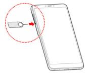
Pull out the card tray. You can place a nano-SIM card on the right card slot, and place a microSD card on the left card slot, as shown. Carefully slide the tray back into place.
