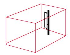
The signals from mobile telephony sector antennas form a rectangular exclusion zone which extends above, below and behind the antenna as well as to the front and sides.
