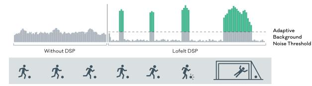
Noise reduction enhances the impact of key events while preventing background noise from vibrating the actuator.
