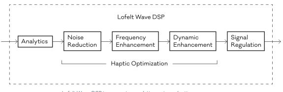
Lofelt Wave DSP incorporates analytics, noise reduction, frequency enhancement, dynamics enhancement and signal regulation components for real-time signal flow optimization.
