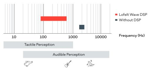
An example of audio events at 2000 Hz being processed into the key haptic sensitivity frequency range.
