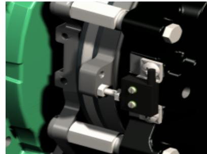
For brakes fitted with a release indicator, while the brake is supplied with power the armature actuates a microswitch (discrete) fixed on the yoke indicating brake release. When the power is switched off, the microswitch changes state in order to confirm that the brake is engaged.
