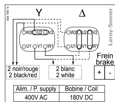
**⚠️** This option is not compatible with motors for operation on a drive. It is not compatible with separate brake power supply (and built-in power supply on two-speed motors).
