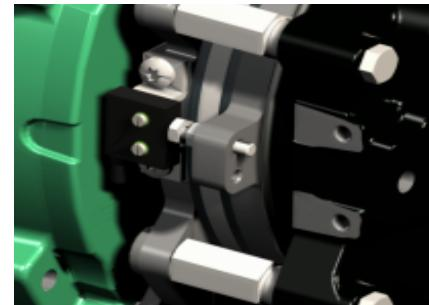
For brakes fitted with a wear indicator, if the brake lining is worn (+ 0.6 mm) the armature actuates the microswitch (discrete) fixed on the backplate and informs the user of the need to adjust the air gap or change the brake lining if it is less than the required minimum.
