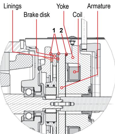
1: air gap with coil energized, brake released
