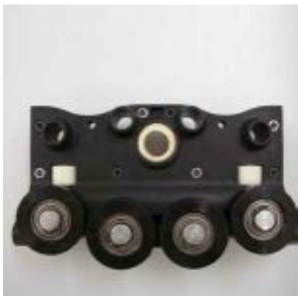
Carriage in a crane system
