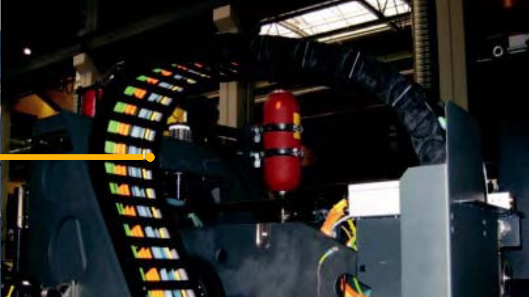
The E4.42 Series in a machine tool, completely assembled with igus® chainflex® cables
