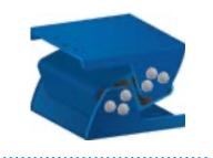
CAB Suspension: The combined characteristics of a spring, a pivot bearing and a vibration/shock damper provide a unique solution for cab suspension. Installation of 4 elements offers parallelogram suspension geometry with a short "X" movement. Minimal "Y" movement provides a very high "side-to-side" stability.
