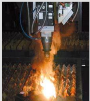
Material load test - laser beam path and burning behaviour
