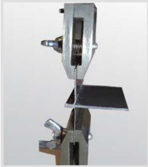
Material load test - tensile test on textiles and strips
