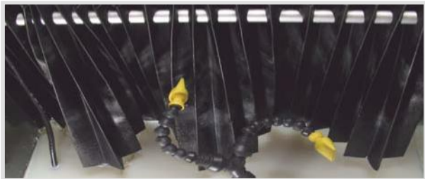
Material load test - coolant spray test, rotating nozzles
