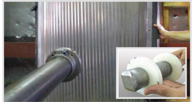
Impact test on covers under DIN EN 12417
