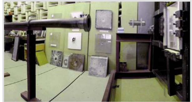
Impact test on safety screens under DIN EN 12415
