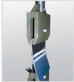
Material load test - tensile test on textiles and strips
