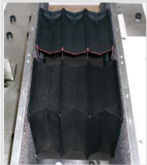
Material load test - flex fatigue strength at the corners of bellows
