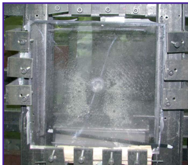
Fixed polycarbonate pane after impact test
