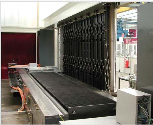
Traverse test on a slat cover with shearing system at the PTW: force sensors measure the vibrations during traverses to block size.
