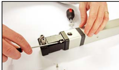
Tighten motor mounting screws
