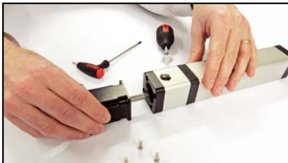
Insert motor shaft into coupling
