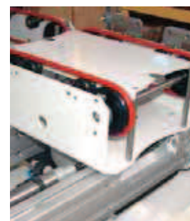
Picture 38.1: Handling- and transportsystem for Semiconductor-Carrier/-Box. The complete system is suitable for the use in cleanrooms, lubrication- and maintenance-free
