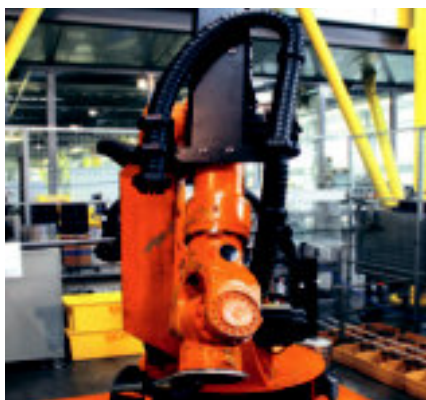
Integrated recuperating spring prevents loop formations
