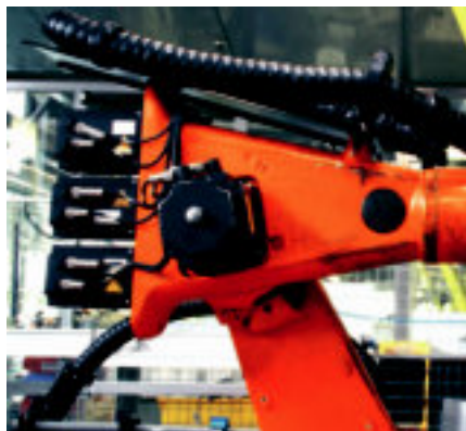
triflex® RS - Extremely flat design, guides close to the robotic arm
