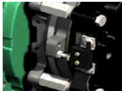
For brakes fitted with a release indicator, while the brake is supplied with power the armature actuates a microswitch (discrete) fixed on the yoke indicating brake release.
