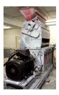
**Grinding** is a key operation in the feed industry process and as such must be reliable. The system has to be flexible to deal with different size reduction requirements while delivering the highest product quality and minimizing fines rate to optimize productivity. Energy consumption is a concern because it is a major part of the operational cost.
