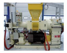
**Extrusion** is a continuous process used in industries such as rubber & plastics, food and feed. Screw extruders' energy consumption is significant and key, it is mostly related to the main drive system.
