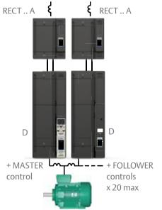
Paralleled inverters allow systems of up to 2.8 MW / 4,200 hp
