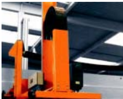
U-shaped supported e-tube for high lateral acceleration
