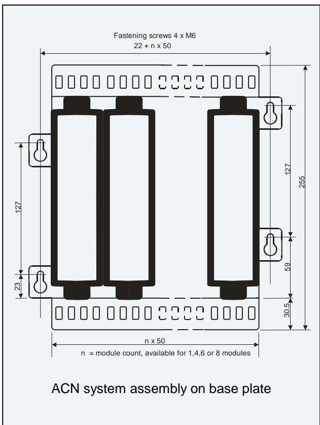
ACN system assembly on base plate
