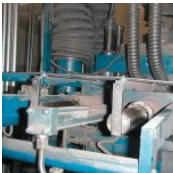
Filling-shoe mechanism in a compaction unit
