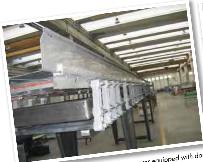
Two-mass shaker conveyor for the transport of bulk material equipped with double rocker arms AD-P 50
