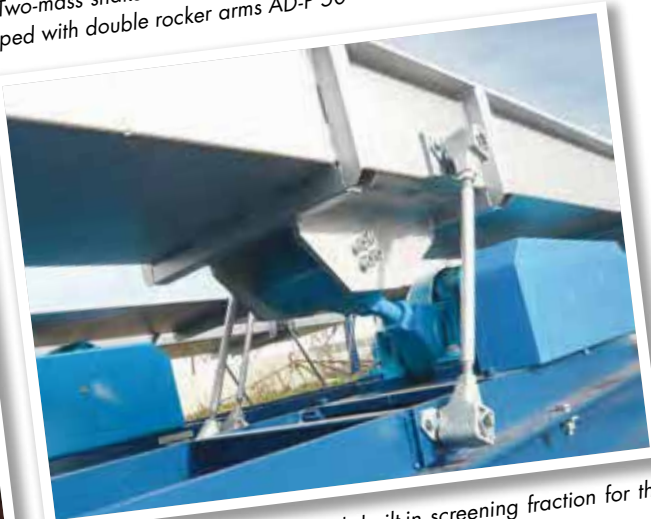
Two-mass "natural frequency" shaker conveyor equipped with double rocker arms made out in light metal casting
