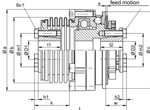
Dimensions [mm]: length dimensions according to DIN ISO 2768 cH
