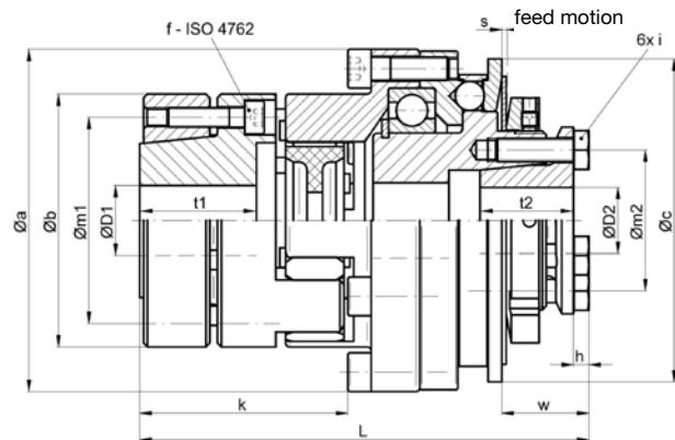
Dimensions [mm]: length dimensions according to DIN ISO 2768 cH
