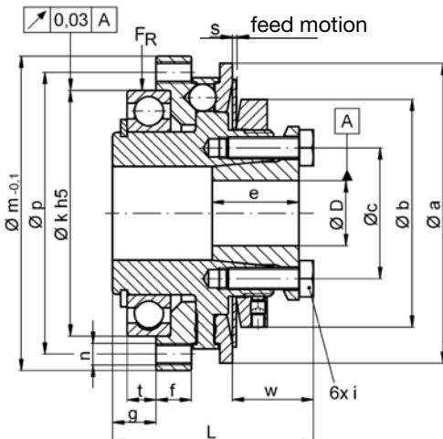
Dimensions [mm]: length dimensions according to DIN ISO 2768 cH
