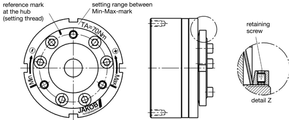
Unscrew retaining screw (see detail Z) completely; turn adjusting nut with pin wrench; after adjustment, secure the adjustment nut against turning by drilling and tightening the retaining screw.
