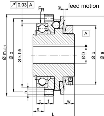
Dimensions [mm]: length dimensions according to DIN ISO 2768 cH
