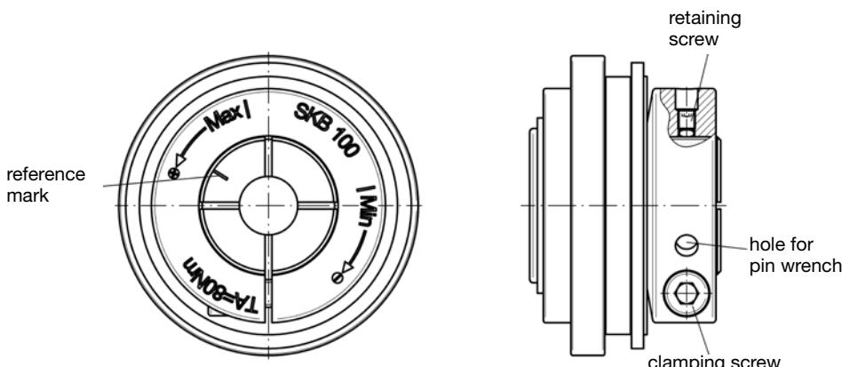
Release retaining screw. Turn adjusting nut with pin wrench (note reference mark). Tighten retaining screw on hub after setting the required disengagement torque. Setting can be done by turning the hub with scale till the required torque value is in line with the reference mark. In mounted state, the clamping screw must be released, and after setting the disengagement torque, it has to be fastened again.
