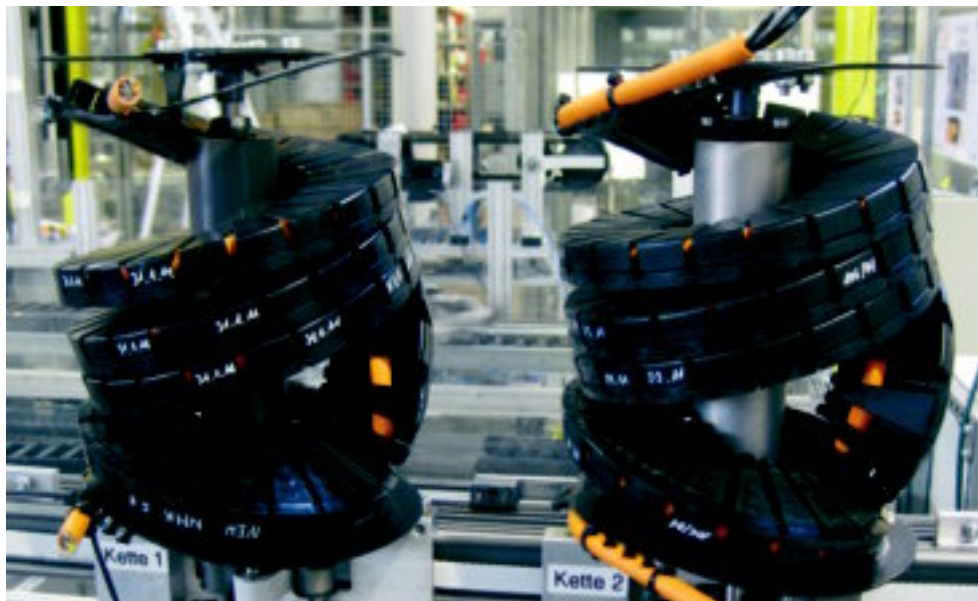
Endurance test of a twisterband module in the igus® test laboratory
