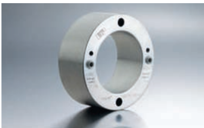
This ETP-AXPRESS is used for fastening and centering of a cylinder in a printing machine for beverage cans of aluminium. It has two separate pressure chambers, one for expansion to the shaft and one to the bore of the cylinder. The runout is better and downtime much shorter than with the mechanical clamping used before
