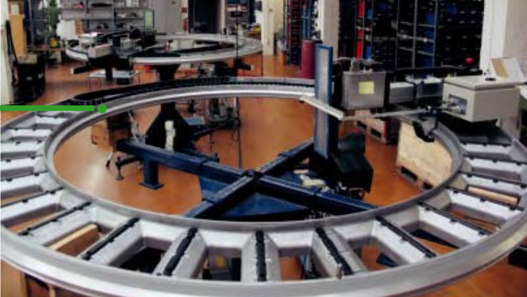
E2 mini e-chain®, RBR-version with reverse bending radius
